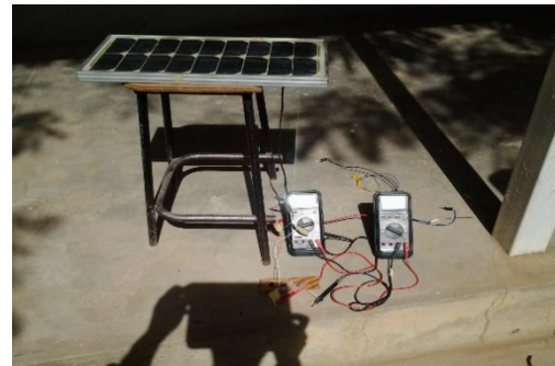
Figure 10: Experimental set-up of the DC-DC converter with PV panel.
